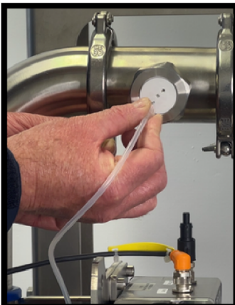
INSERT NEEDLE INTO UNUSED SEPTUM PORT
