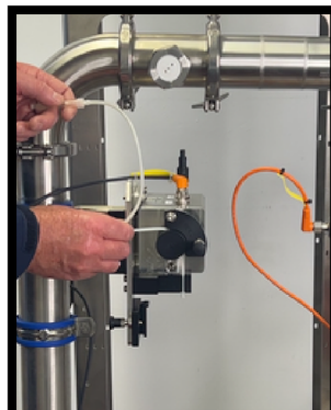
UNCLIP THE TUBE FROM THE SAMPLER
